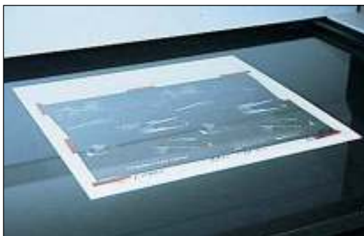
LITHOPROOF IN EXPOSURE FRAME
