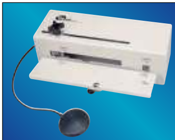
Lower guide comb and insert UniCoil® into feed for simple automatic insertion.
