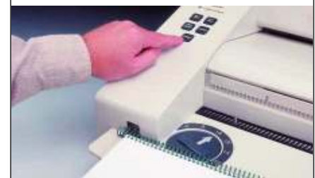
Finish the process with a powered crimp/cut on both ends of the UniCoil-bound document.
